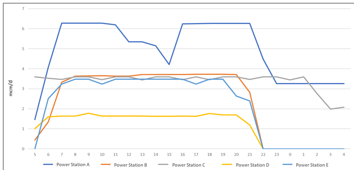
Figure 13 South West power station flow profile over a real gas day in 2020
