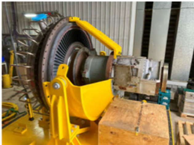
Figure 48: [redacted] 2A - HSPT assembly removal and installation into shipping container
