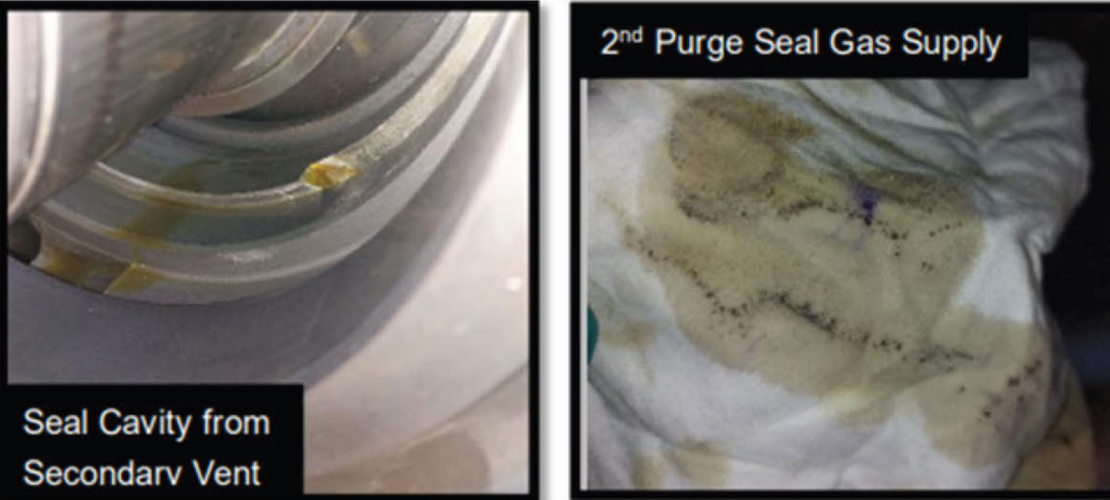
Figure 38: [redacted] Unit B Dry Gas Seal – Seal cavity had presence of oil on removal of DGS, behind both the Inboard and outboard positions. To clean casing lines appropriately 5 Bar of Nitrogen was introduced, and a white cloth covering the other end, purging until clean
