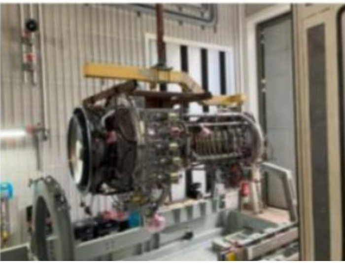
Figure 45: [redacted] Unit 2A - Gas generator removed from container and installation in package in process
