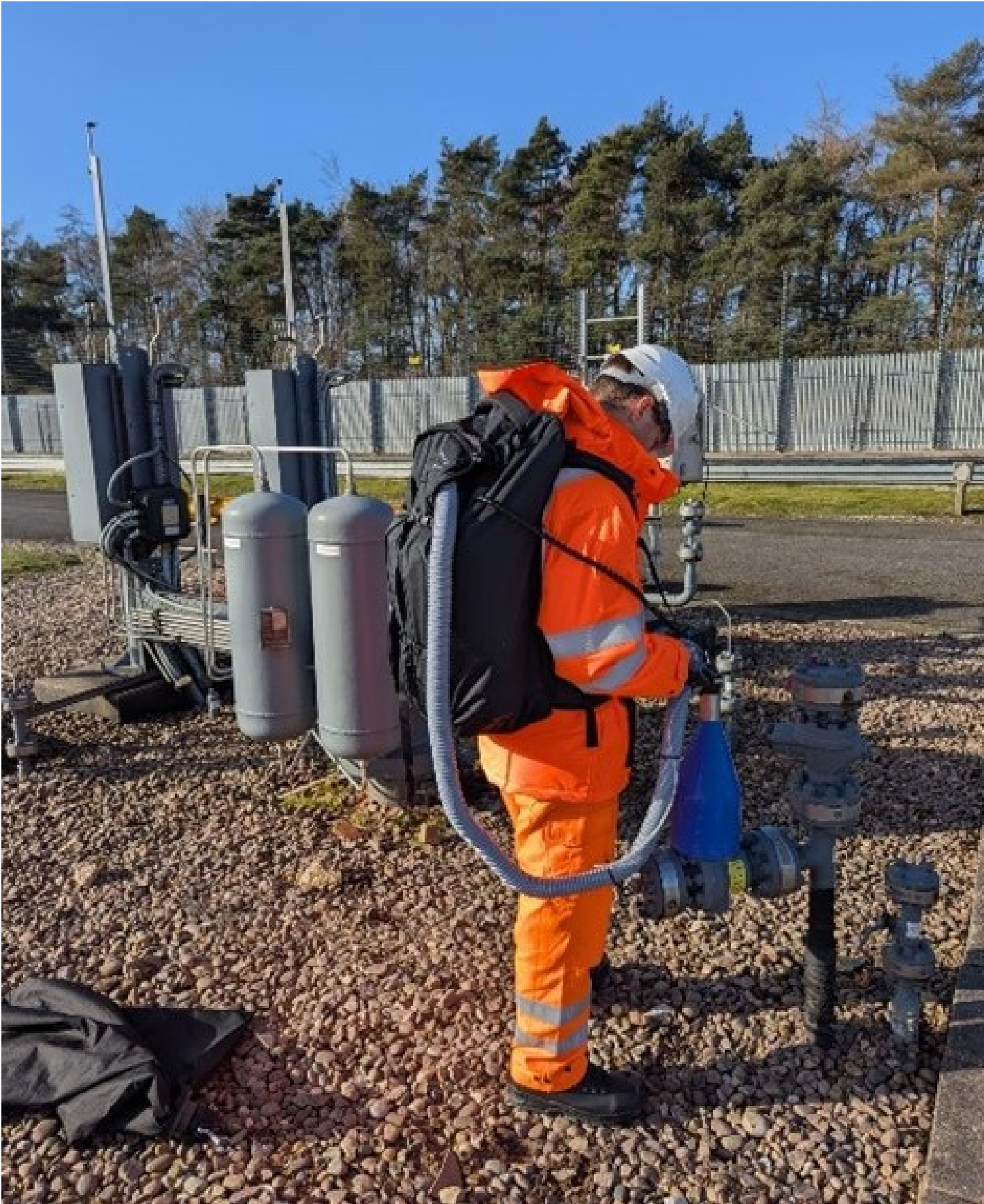
Figure 32: Example of ground level accessible fugitive leak quantification by HiFlow sampler
