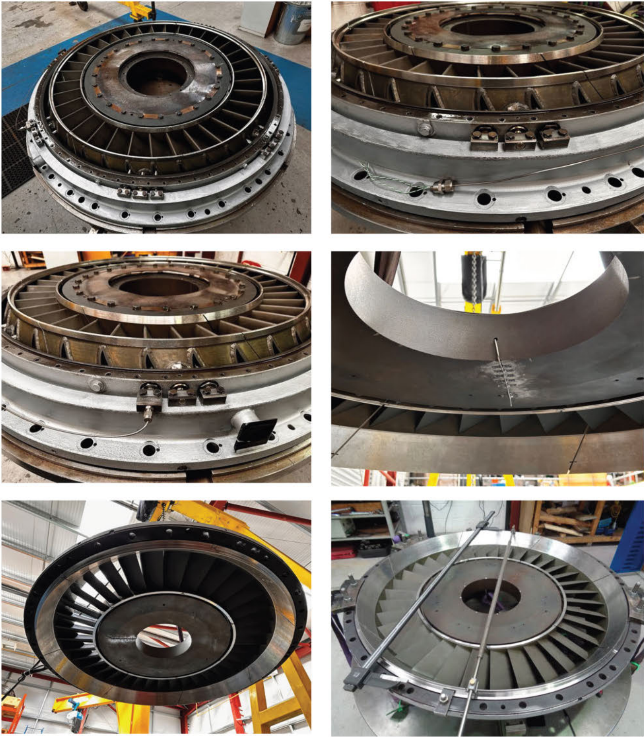
Figure 52: [REDACTED] B - Nozzle was re-assembled with new set of nozzle segments, cooling air pipes (welded into position) all new consumables, locking plates, sealing strips and a new T/C stitch welded in place.
