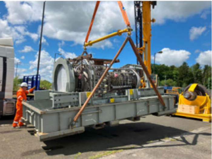
Figure 43: [redacted] 2A - Inspection of new gas generator in container before being transported to package
