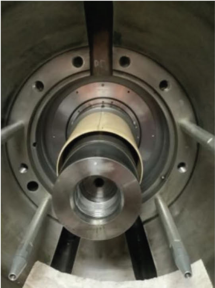
Figure 41: ██████████ Unit 2A - DGS ports borescope and liquids drained before being installed
