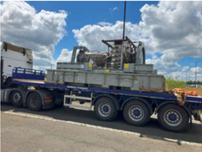
Figure 43: [redacted] 2A - Inspection of new gas generator in container before being transported to package
