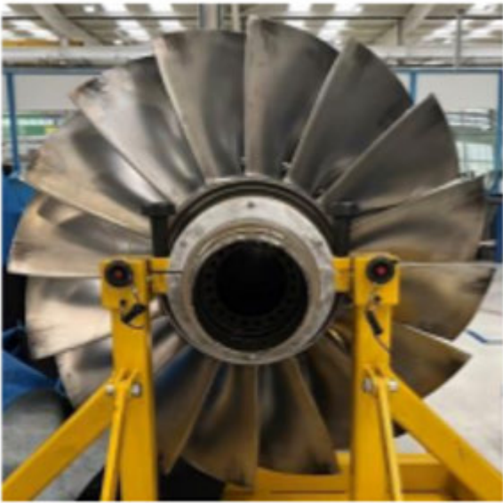
Image 28: XXXXXXXXXX LM2500 Gas Generator Overhaul - Inspection of the high-pressure compressor rotor blisk, assessing blade condition, integrity and wear to support refurbishment and ensure liable in-service performance.
