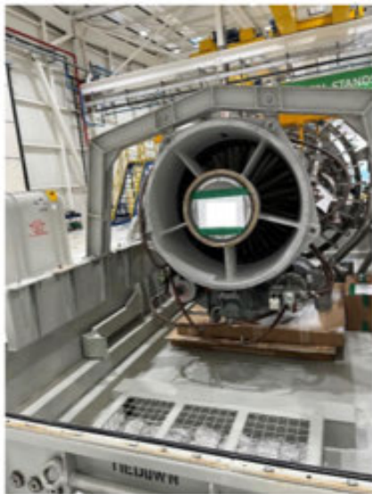
Image 33: [REDACTED] LM2500 Gas Generator Overhaul - Fully overhauled unit following inspection, refurbishment and reassembly, ready for return to service.
