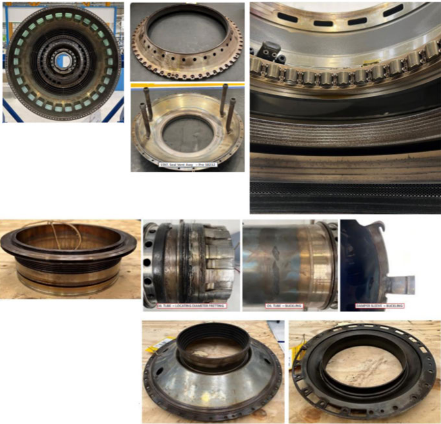
Image 30: XXXXXXXXXX LM2500 Gas Generator Overhaul - Inspection of compressor rear frame components, assessing wear, sealing surfaces and structural condition to inform refurbishment and ensure integrity on return to service
