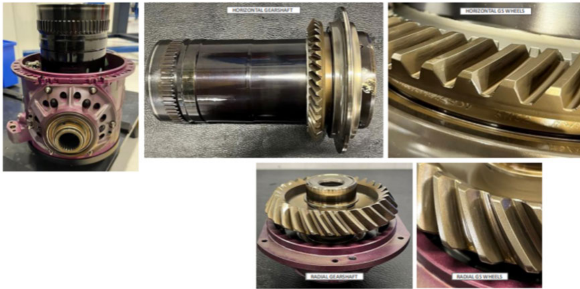
Image 31: [REDACTED] LM2500 Gas Generator Overhaul -Inspection of the inlet gearbox assembly, including shafts and gear wheels, assessing wear, alignment and component condition to ensure reliable power transmission on return to service
