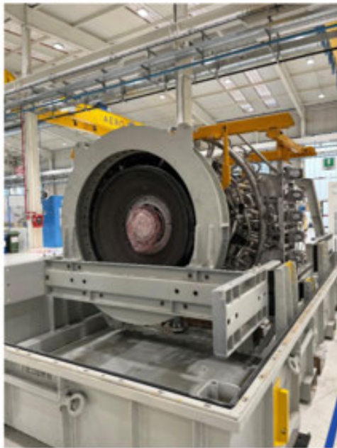
Image 33: [REDACTED] LM2500 Gas Generator Overhaul - Fully overhauled unit following inspection, refurbishment and reassembly, ready for return to service.
