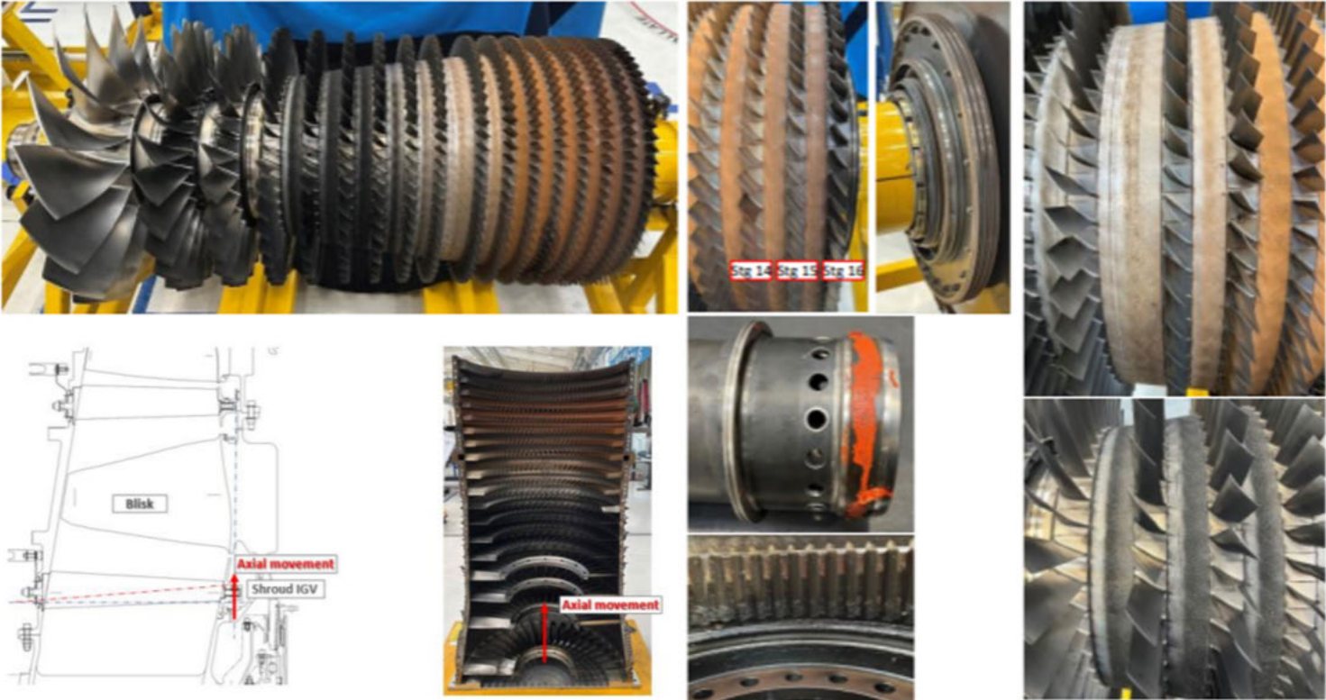
Image 27: XXXXXXXXXX LM2500 Gas Generator Overhaul - Detailed inspection of the high-pressure compressor roto and blisk assemblies, assessing wear, fouling and axial movement to inform refurbishment and ensure reliable performance on return to service
