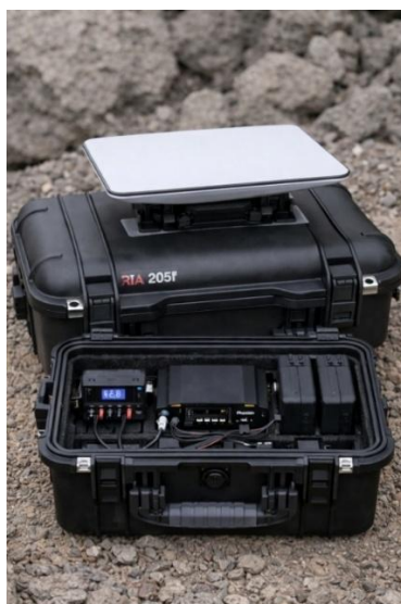
Figure 3: Example of Peli case based deployment solution – Operational deployment.
