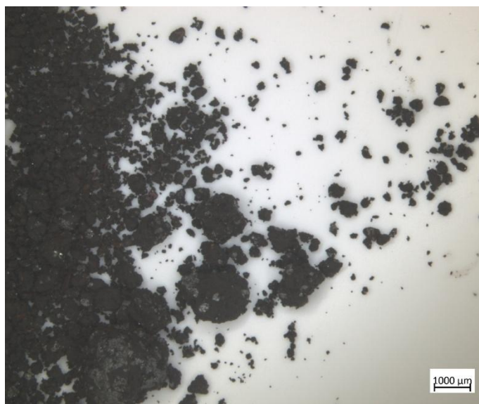
Figure 18 Sample [REDACTED] stereo microscopic image showing smaller particles of metallic material.
