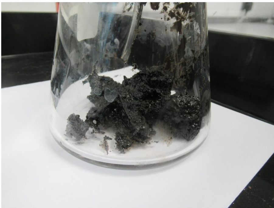
Figure 85 Sample [REDACTED] one hour into the hydrogen exposure testing.
