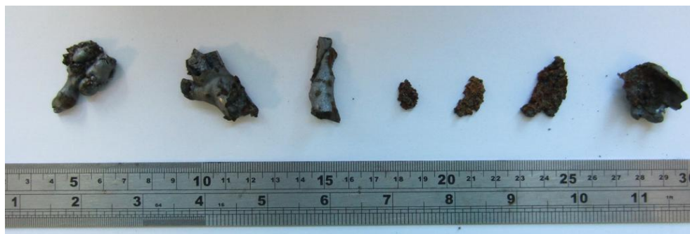
Figure 38 Sample [REDACTED] weld spatter showing varying levels of contamination.
