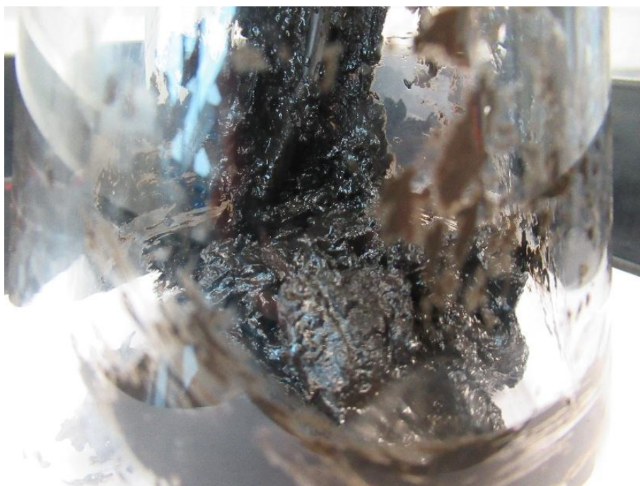
Figure 93 Sample [REDACTED] halfway through the hydrogen exposure testing.
