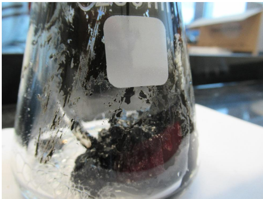
Figure 79 Sample [REDACTED] three hours into the hydrogen exposure testing.
