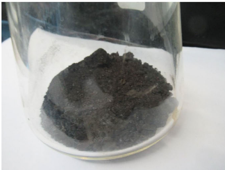
Figure 108 Sample [REDACTED] three hours into CO 2 exposure testing.
