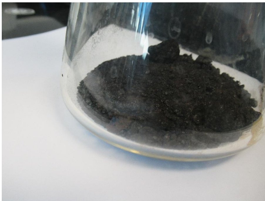
Figure 99 Sample [REDACTED] halfway through CO 2 exposure testing.
