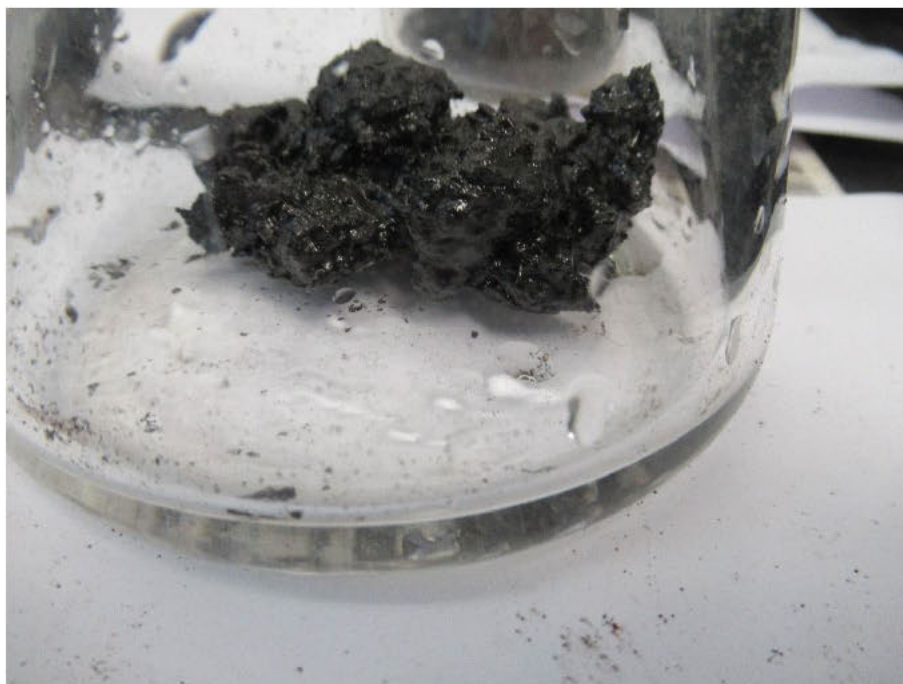
Figure 124 Sample [REDACTED] at the end of the CO 2 exposure testing.
