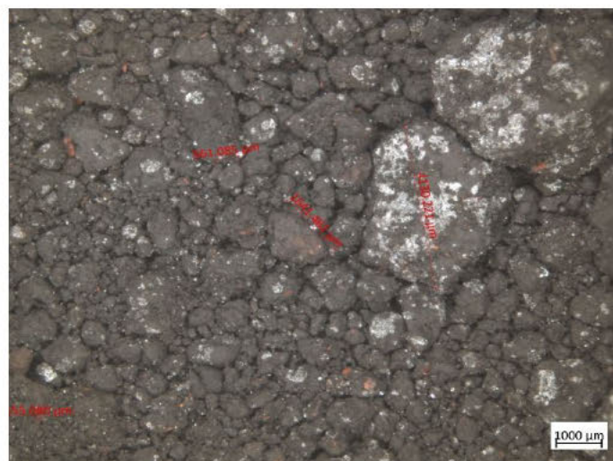
Figure 16 Sample [REDACTED] stereo microscopic image showing varying sizes of metallic particles.
