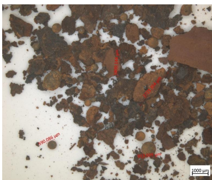
Figure 32 Sample [REDACTED] stereo microscope image of smaller particles including spherical particles likely to be weld spatter or shotblasting material.
