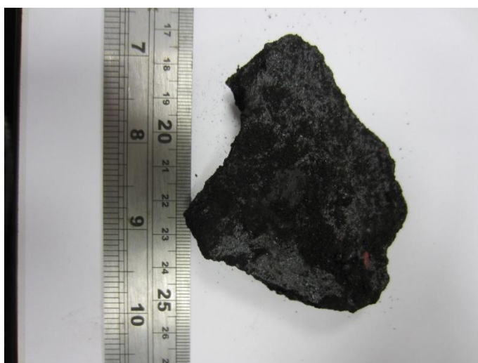
Figure 14 Sample [REDACTED] solid material with black dust-like contamination.
