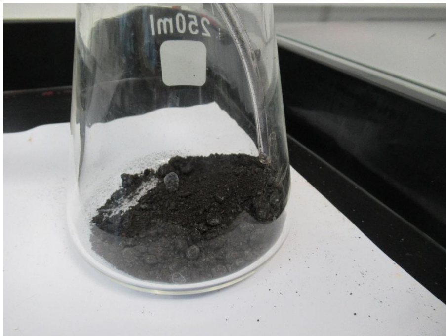
Figure 60 Sample [REDACTED] after one hour of hydrogen exposure testing.
