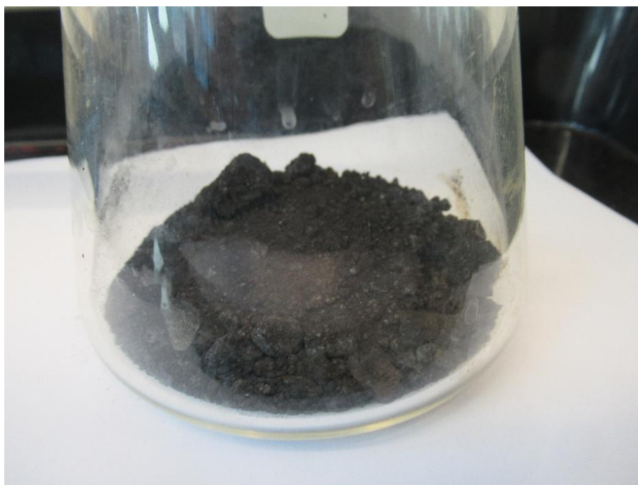
Figure 98 Sample [REDACTED] after one hour of CO 2 exposure testing.
