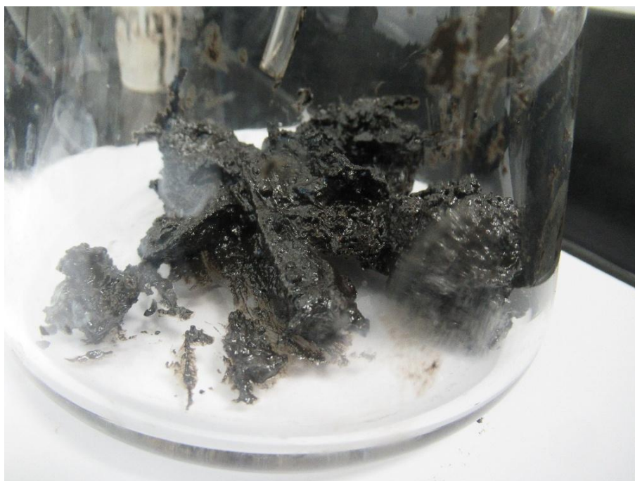
Figure 88 Sample [REDACTED] at the end of the hydrogen exposure testing.
