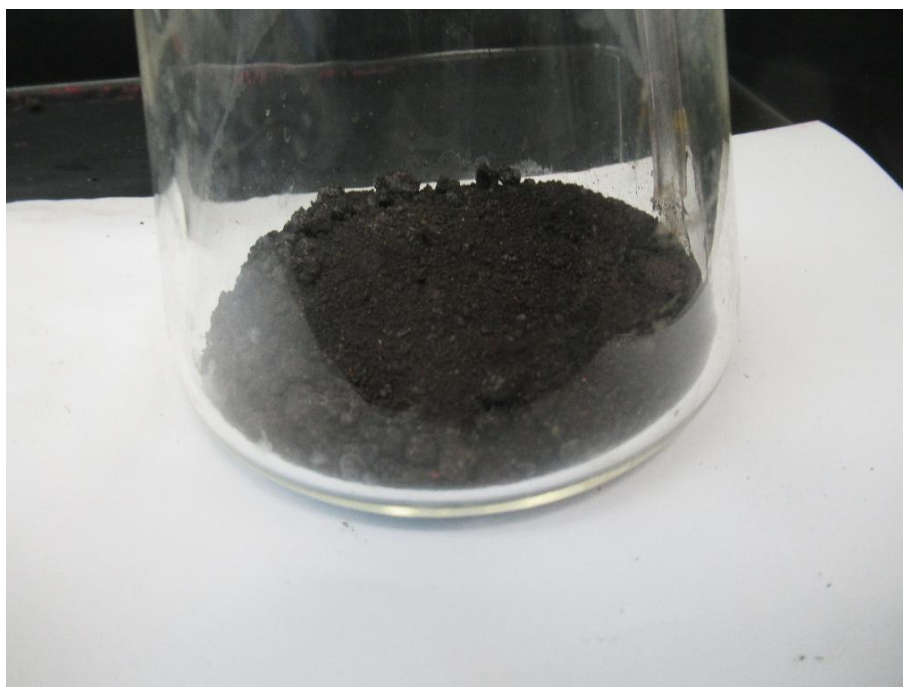
Figure 73 Sample [REDACTED] at the end of the hydrogen exposure testing.
