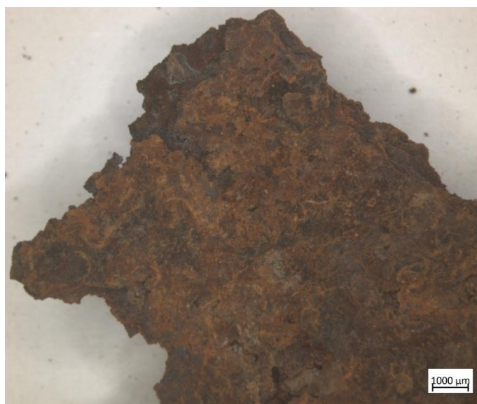
Figure 31 Sample [REDACTED] stereo microscope image of pipe scale.
