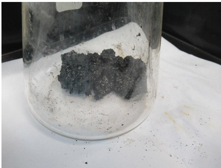
Figure 135 Sample [REDACTED] halfway through the CO 2 exposure testing.
