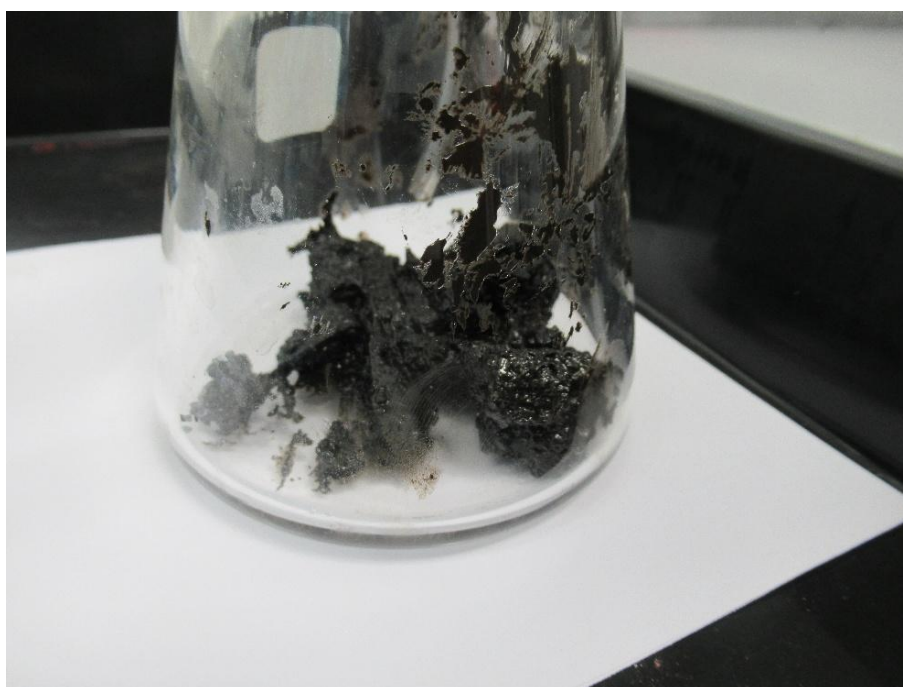
Figure 87 Sample [REDACTED] three hours into the hydrogen exposure testing.
