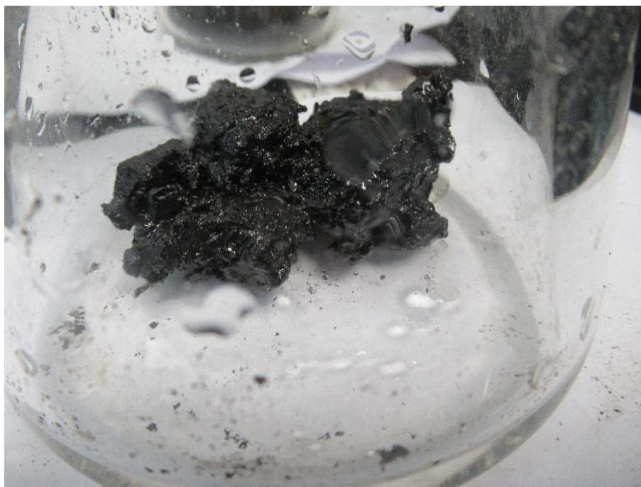
Figure 123 Sample [REDACTED] halfway through the CO 2 exposure testing.
