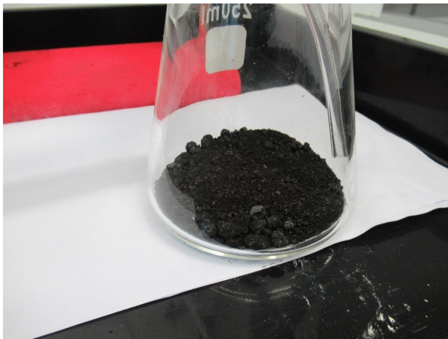
Figure 53 Sample [REDACTED] three hours into the hydrogen exposure testing.
