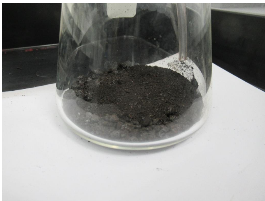
Figure 70 Sample [REDACTED] after one hour of hydrogen exposure testing.
