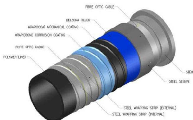
Figure 25 MASiP pipe structure
