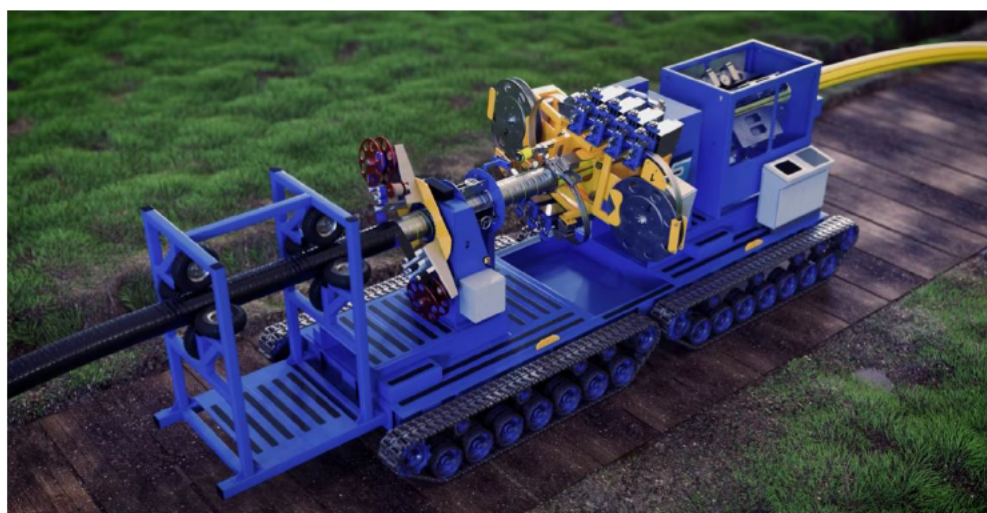
Figure 26 MASiP pipe mobile fabrication concept
