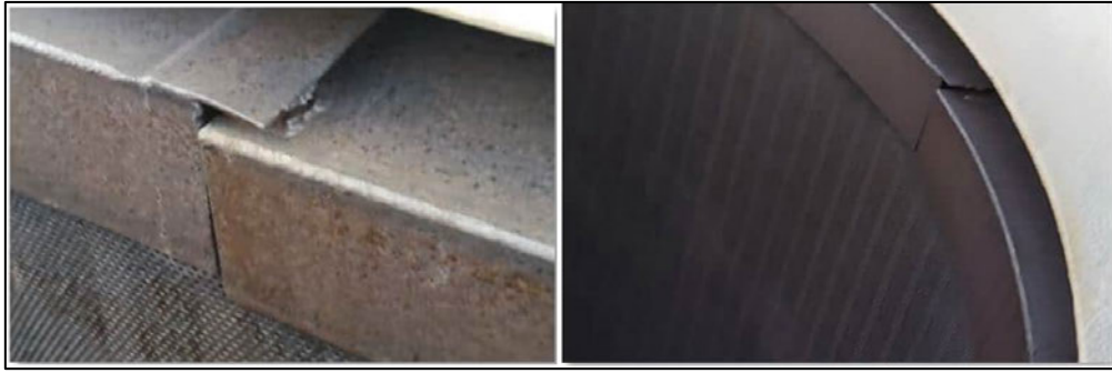
Figure 24: Unit 1A Exhaust and bullet: Pictures show broken weld in the cowl
