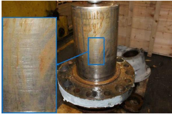
Figure 2: Leaking stem due to wear
