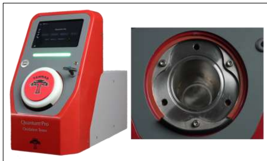
Figure 1: Tannas & King Quantum Pro High Pressure Oxidation Vessel
