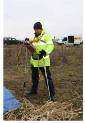
MC Miller Candidate device with prototype AC CIPS module and measurement probes attached during field trail at Stallingborough power station
