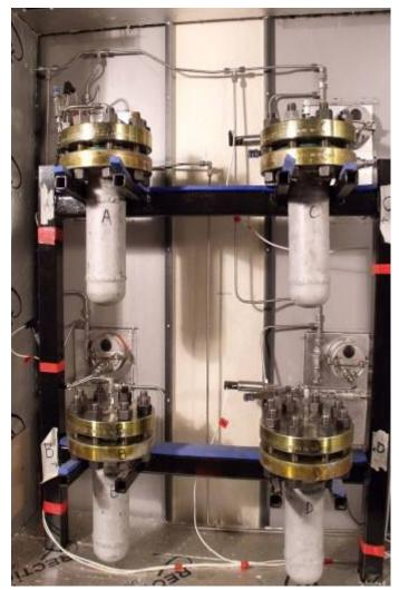
Figure 1 Corrosion test rig arrangement
