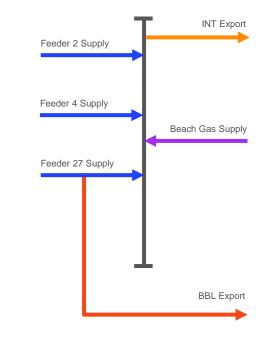
Simplified schematic of Bacton pipework arrangement
