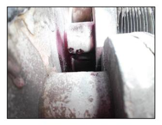
Figure 16 Tube Bundle Header Connection Through Wall Defects
