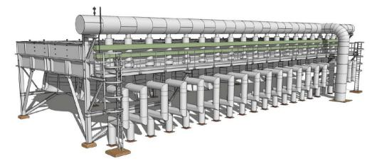
Figure 5: General Aftercooler Diagram
