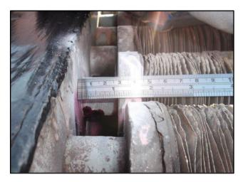
Figure 15 Tube Bundle Header Connection Through Wall Defects
