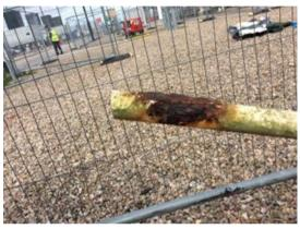
Figure 9: Through wall corrosion requiring replacement to continue operation
