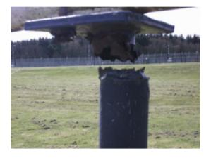
Figure 8: Damaged pipe support through corrosion and movement
