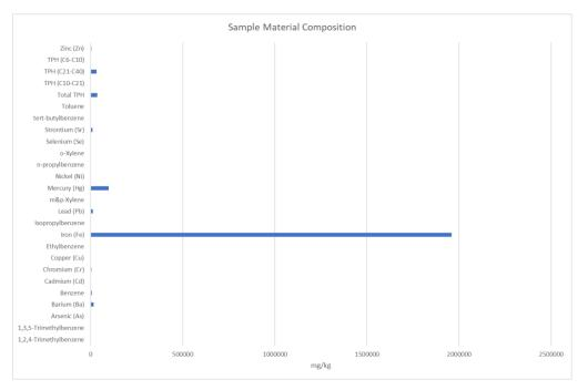
Figure 8: Filter Maintenance Material Sample Chemical Analysis
