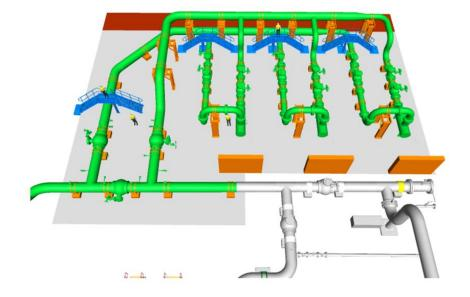
Figure 36 3D Model of Feeder 4 Filter Pipework Arrangement
