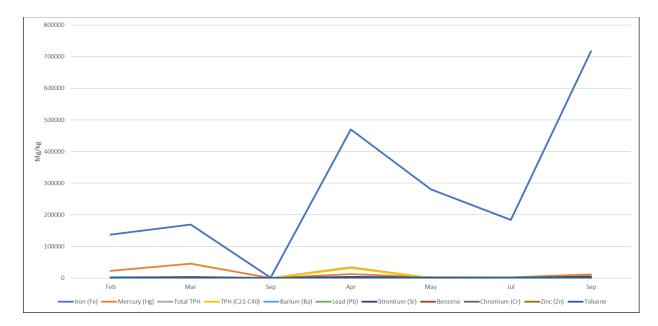
Removing iron from the graphs provides better granularity of the other elements identified. A range of other elements were generally identified within the samples, including Mercury, TPH (Total Petroleum Hydrocarbons), Barium, Strontium. These elements are generally found with gas composition and are a by-product of the extraction.
