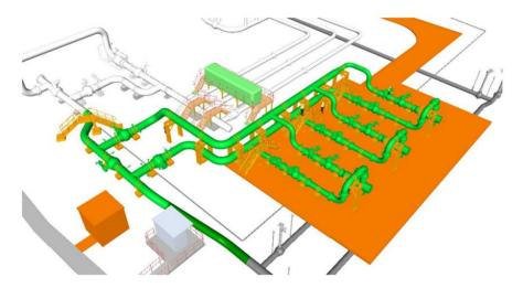
Figure 37 3D Model of Feeder 4 Filter Pipework Arrangement
