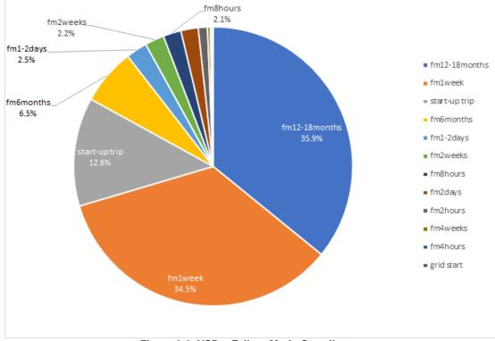
Figure 3-9, VSD – Failure Mode Contributors
