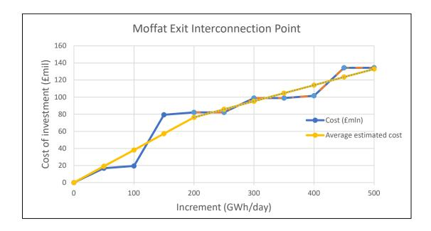
N.B. The main reason behind the estimate being considerably lower at Moffat Interconnection Point is that no new pipeline reinforcement was required in the analysis undertaken to accommodate the additional demand at that Exit Point.
