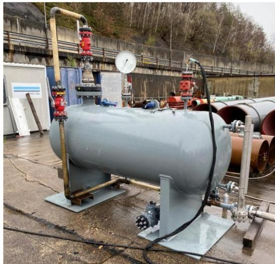
**Figure 4: Mobile condensate storage tank.**
