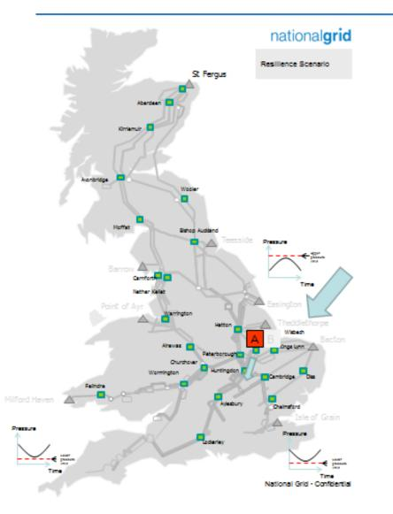
Wisbech compressor was originally built to support southern pressures and maintain pressures below safe operating limits at Easington and Theddlethorpe supply terminals
