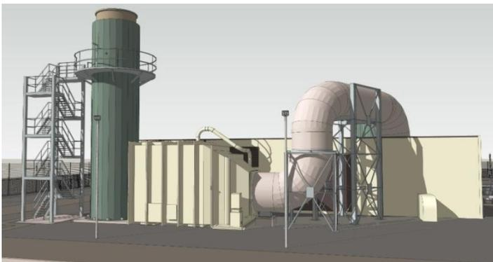
Figure 7: Compressor cab with SCR fitted
