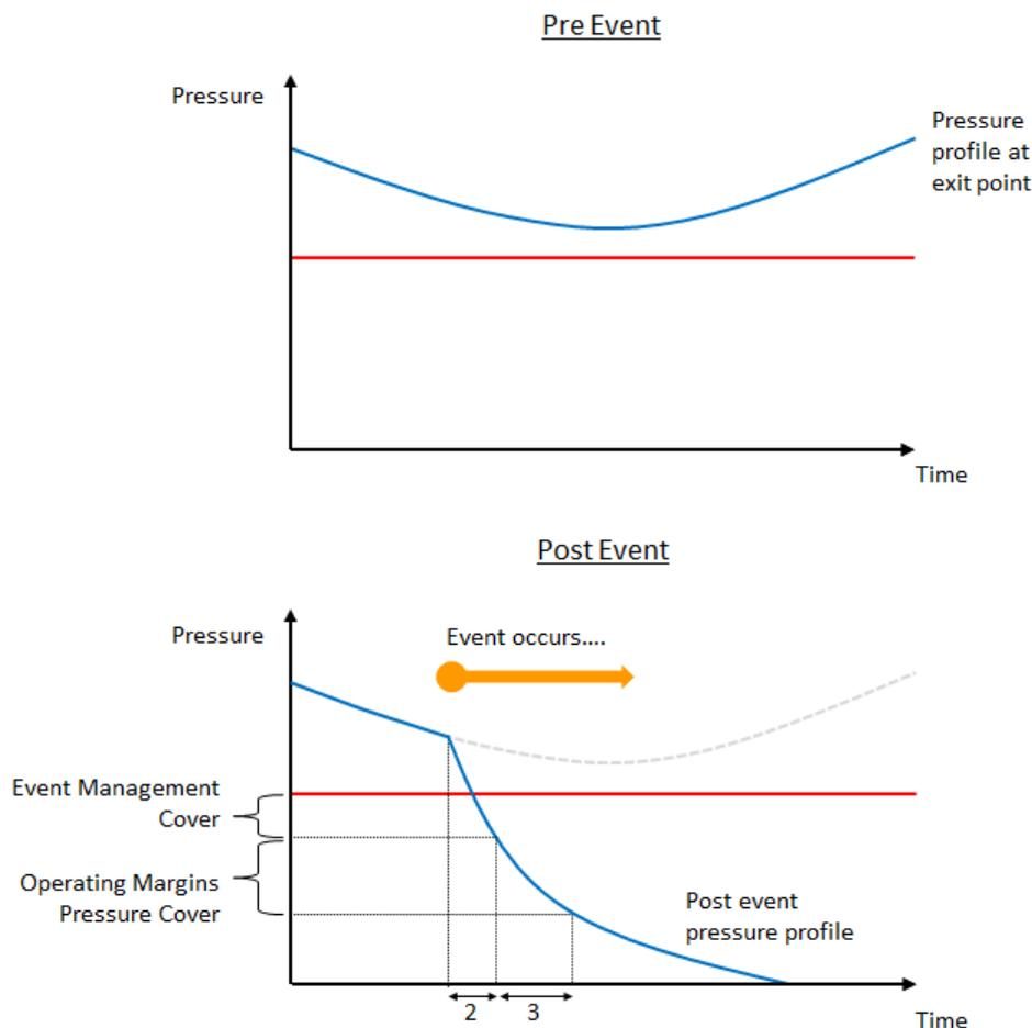
Figure E10: Calculating pressure cover
